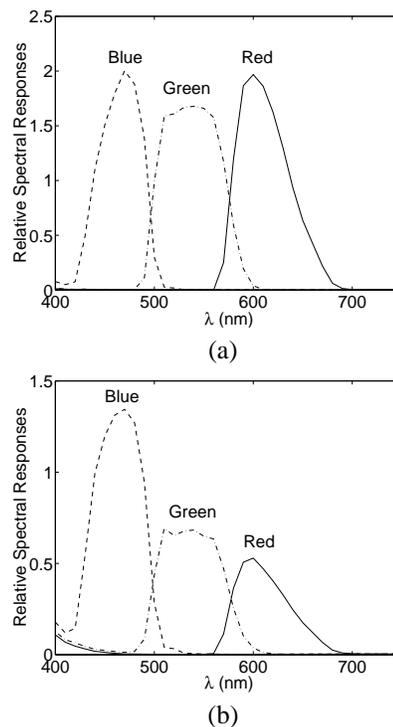
Figure 7: Spectral sensitivity curves for the camera characterized with an objective. These were obtained by scanning the spectrum at  $10\text{ nm}$  intervals between  $400\text{ nm}$  and  $700\text{ nm}$ . In (a) color balancing has been performed, whereas this is not the case in (b) where the curves are those of the factory settings.
