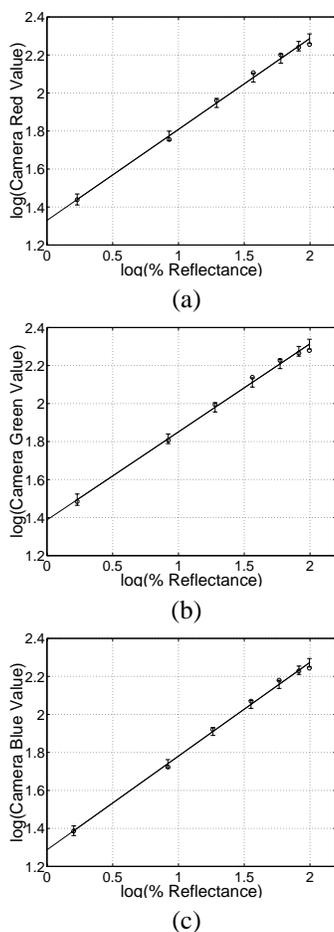
Figure 3: Log-log plots for obtaining the gamma parameters of the camera for the (a) red, (b) green, and (c) blue channels respectively. The lines are least-square fits to the data points, *c.f.* Eq. (6), with error bars showing the estimated errors of the fit at the data points. The data points are within the error bounds of the fit.
